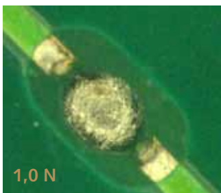
Example: Contacting SAC solder with tip style 02 and various spring forces
