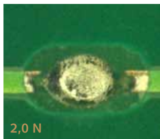
Example: Contacting SAC solder with tip style 02 and various spring forces
