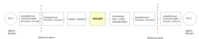
HFS-807 303 051 A 6842 HFM-M, RF measurement setup
