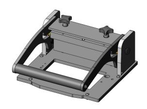
**General data** Product group: Manual drive unit Main series: ATE MAXXX Series: ATE MA2xx Size: 260 Test fixture type: With mounting plate Contact stroke generation: Manual Max. interface signals: 150 Interface blocks required: 300 N [1,079 ozf] Max. contact force: Approx. parallel contact stroke: 15 mm [.59 in] Min. temperature: 10 °C [50 °F] Max. temperature: 60 °C [140 °F] RoHS-compliant:
