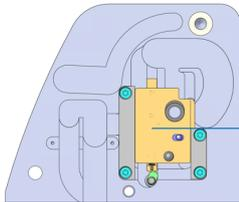
Mechanical 2-stage locking unit without electric motor, for tests without self-opening unit
