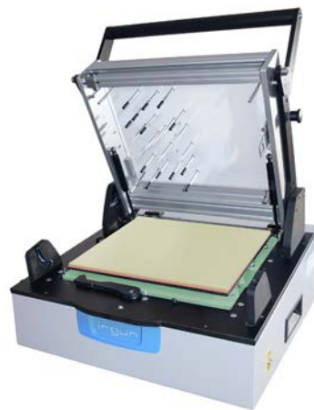
Figure 5: Placement of the thin cleaning mat in a manual test fixture.
