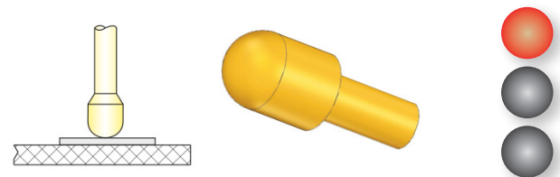
Figure 3: Cleaning mats are not suitable for less aggressive tip styles
