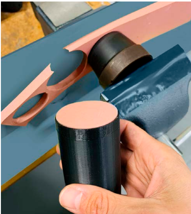
Figure 6: Making an in-situ cleaning cell using contact cleaning mats (1)
