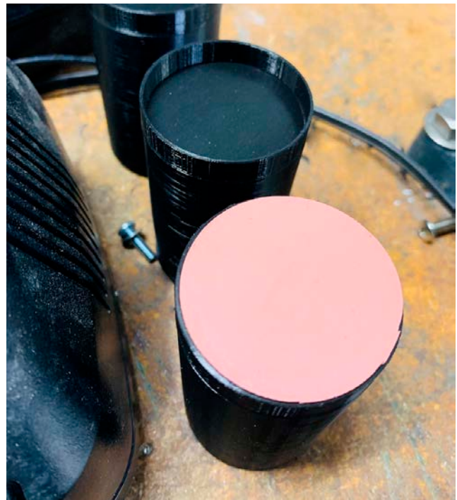
Figure 7: Making an in-situ cleaning cell using contact cleaning mats (2)
