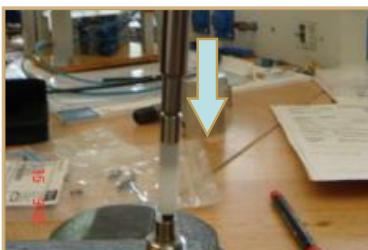
7. Press in the spare parts vertically until friction bearing flush with head of marking unit. Secure the marking head vertically in place to avoid axial strains of the gear motor.
